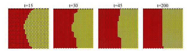
Figure 5. The evolution of a curved grain interface
