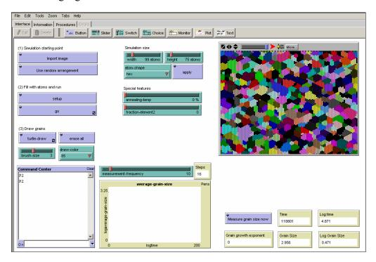
Figure 2. MaterialSim's grain growth model
